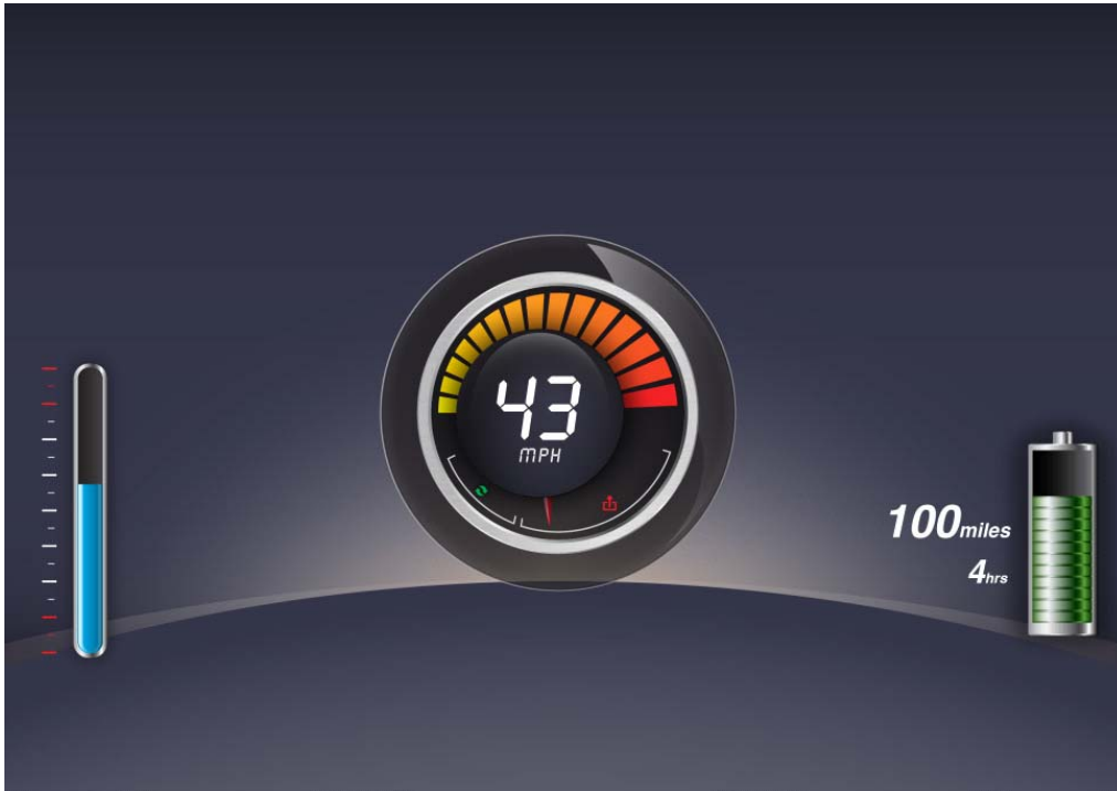
Figure A rough layout to show the place of different instruments on the dashboard for standard user. From Figure 4.8 There is a general image about the position for each instrument on the dashboard, for the standard users. For driving an electric power car, besides the speed information, the battery temperature and the battery status are equally important to know, according to the system study. Because of this, the battery temperature and the battery status gauges are located to the sides of the speedometer, two obvious positions.
