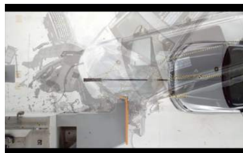
Figure 23. Audi Q7 2017 small overlap test
