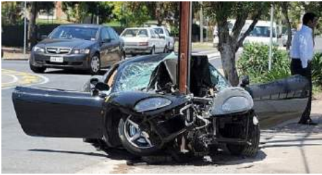
Figure 20. Real examples of a front pole impact
