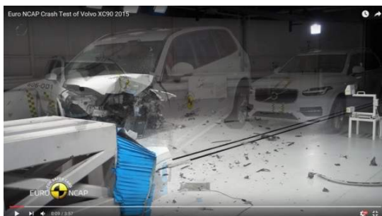
Figure 27. 2016 Volvo XC90 moderate overlap
