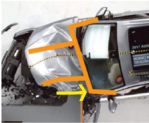
Figure 24. 2017 Audi Q7 small overlap test load path
