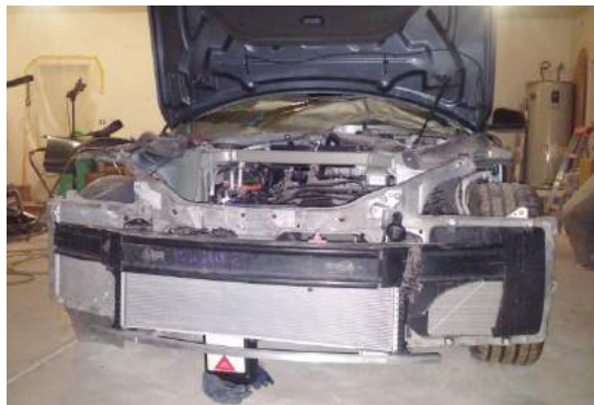
Figure 61. Cooling pack positioning on the Tesla model S
