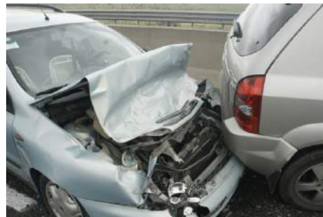
Figure 21. Front to end vehicle incompatibility
