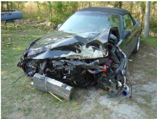
Figure 13. Example of a vehicle impacted on a moderate overlap real situation
