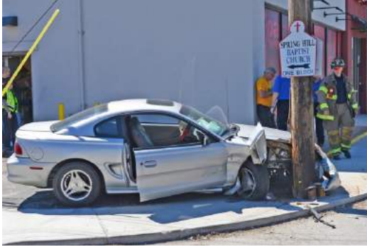
Figure 16. Example of a vehicle impacted by a small overlap real situation
