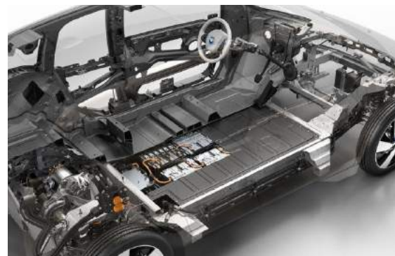
Figure 51. Batteries and firewall
