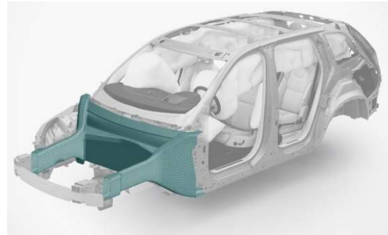
Figure 28. CAD model context of the frontal structure of a XC90
