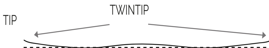
Figure 10. The rocker of the ski is the rise in the tip and tail of the ski
