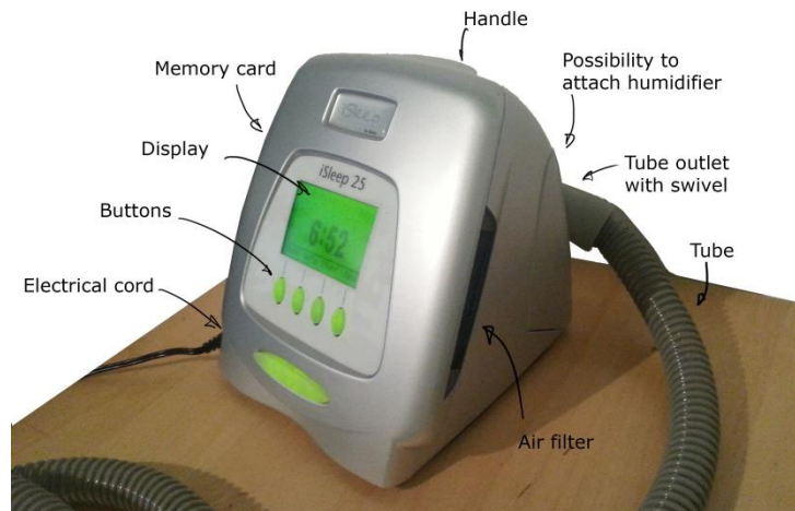
Figure 2 - Common parts of a CPAP device
