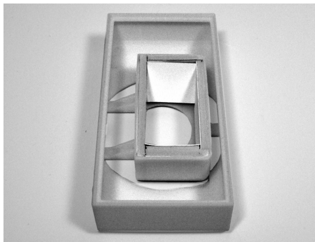
Figure 67. A 3D printed part representing the reflector and housing component surrounding it.
