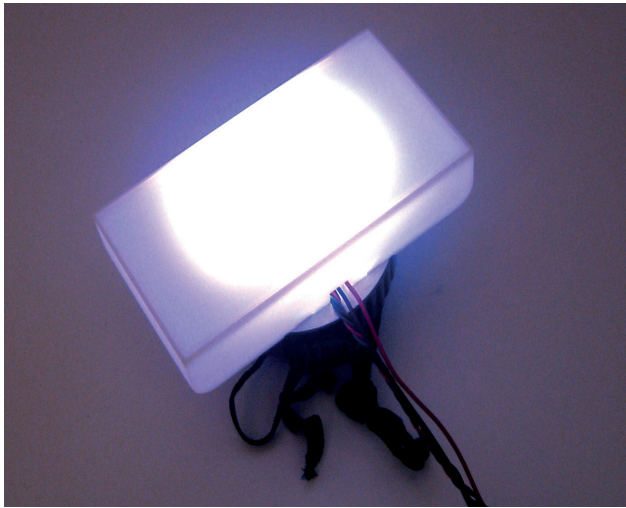
Figure 70. The reflector blocked out some of the light for the light diffuser.
