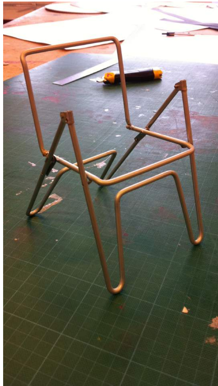
Figure 63. The scale model built to define the final measurements and proportions of the chair.
