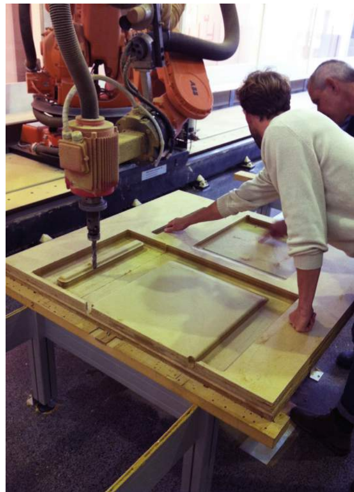
Figure 79. Milling of the felt tooling.
