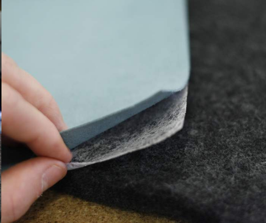
Figure 81. The three components of the felt pressing process. Bottom up: Polyester felt. Polyester glue sheet and Furniture textile
