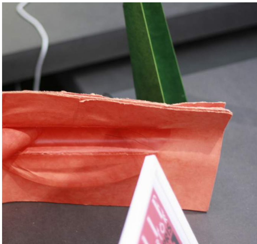
Figure 28. New material Durapulp by Södra. A composite material made from paper pulp and a bio degradable polymer. Assigned a material spur; “Durapulp”
