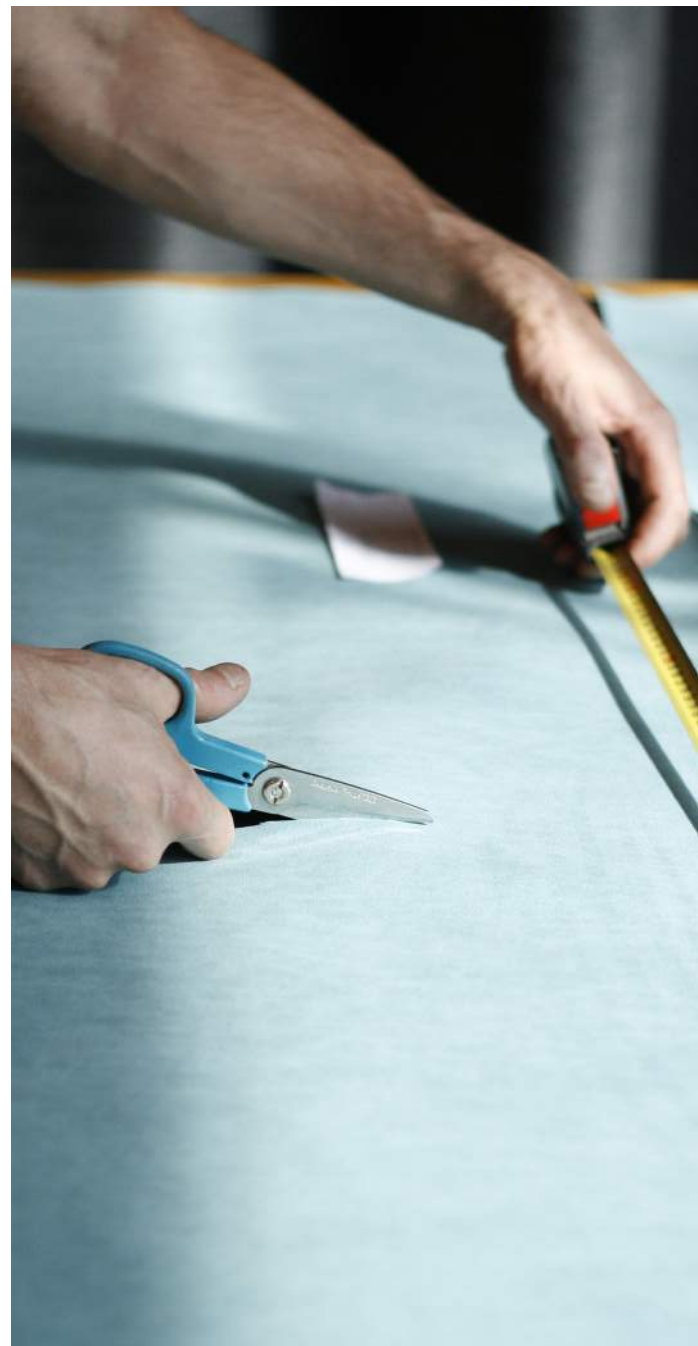
Figure 32. Furniture textile is being cut to the right shape and size before the pressing procedure
