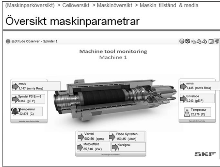
Figure 42: An example of the process media and machine condition parameter visualization
