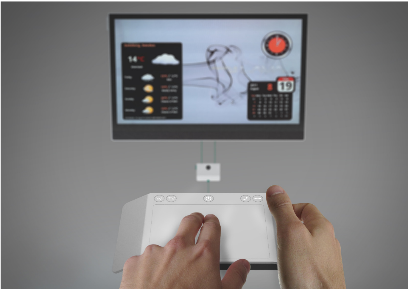
Figure 9.14 The user controls the Window to the World software by moving an onscreen cursor with the trackpad
