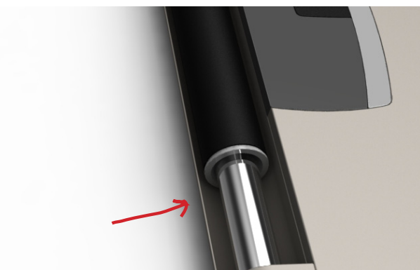
Figure 11.2 The ledge on the backside keeps the roll bar clear from any other objects.
