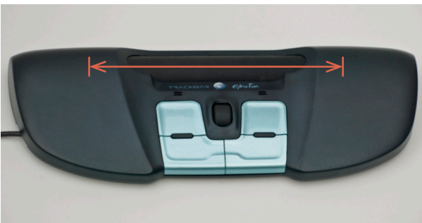
Figure 6.2 The roll bar hits the ends which causes some frustration among the users.
