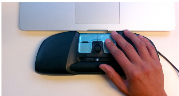
Figure 6.7 The Trackbar can be used backwards, which can be a good feature.
