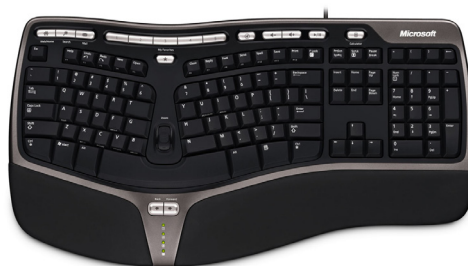
Figure 6.6 An ergonomic keyboard with a curved front make the CPD:s fit badly and cause a distance.
