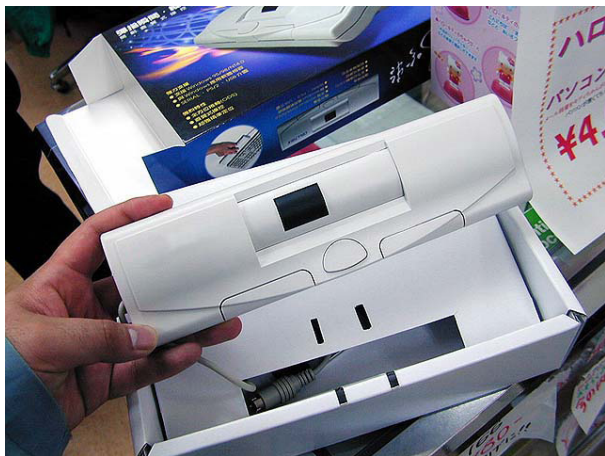
Figure 2.2 The first product, Trackbar Pro, had three buttons and a small roll bar for the cursor control.
