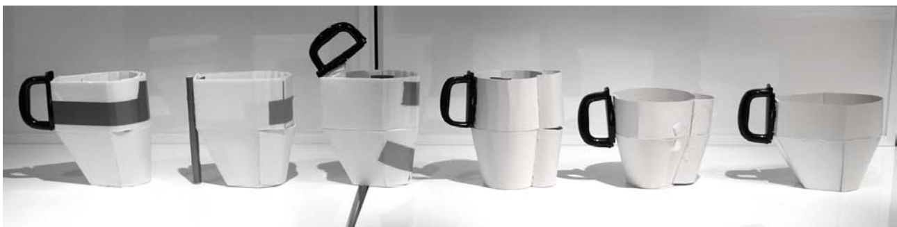
Figure 6.8 Different mock-ups to evaluate the form of the jug
