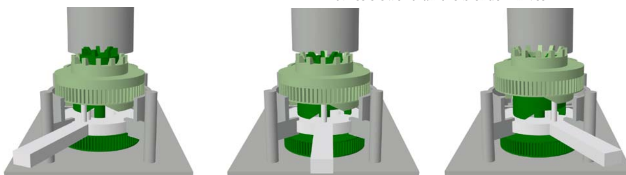
Figure 7.16 The function of the clutch. Pushing the control to the right will cause one of the clutches to go up, while the other clutch will go up when the control is pushed to the left.
