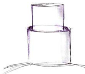
Figure 5.13 Telescopic feeding chute
