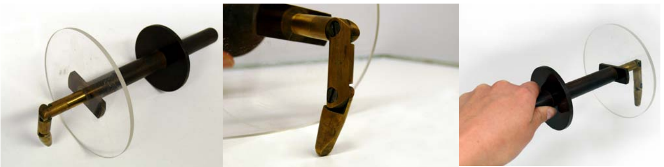
Figure 2.11 A standard probe to ensure safety for the user
