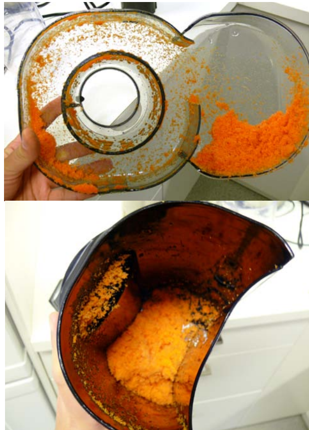
Figure 4.7 A lid and a scrap container from a centrifugal juicer after juicing 200 g of carrot
