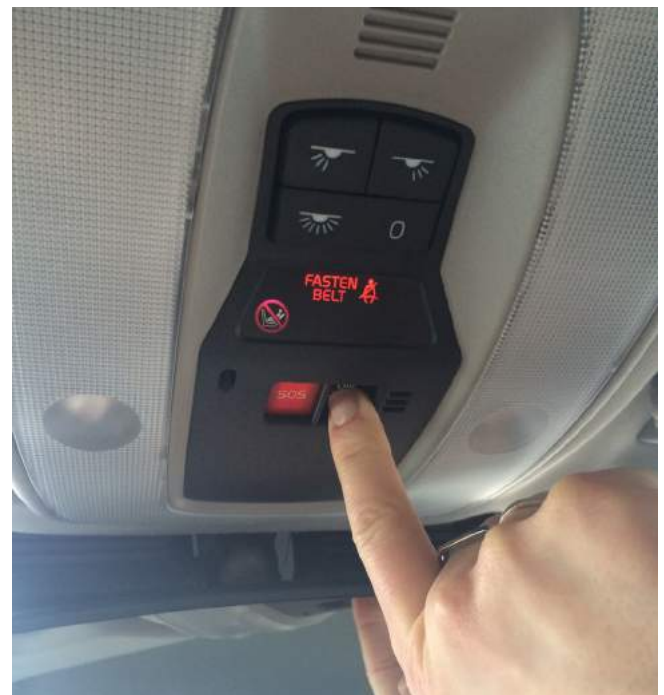
Figure 4B. The driver can reach the call center by pushing one of the hardware buttons, which are integrated in the car's ceiling.
