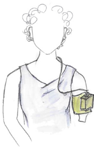
Figure 24. The box worn on the residual limb with ground electrode in the neck.
