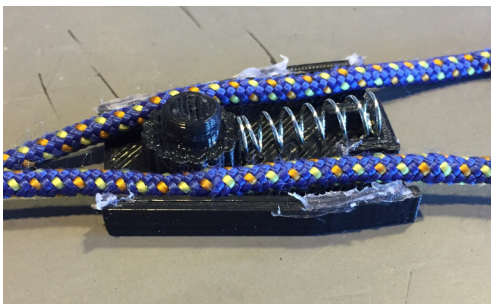
Figure 51. 3D printed cord lock with a nylon string.
