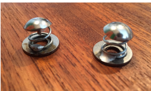
Figure 56. Electrodes made for 8 mm liner.
