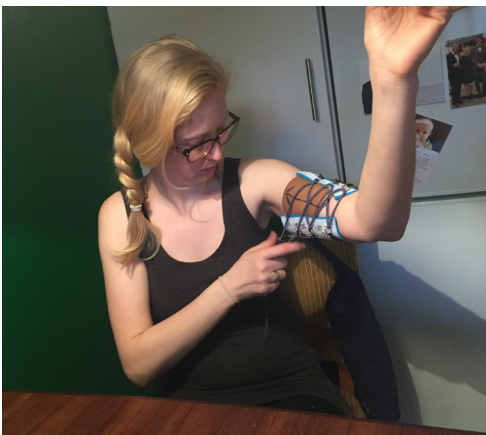
Figure 71. One user does the usability test, that had some problem with the lacing and tightening.
