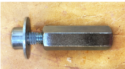
Figure 53. Mock-up of an expandible screw. The right part is the distance nut, which is locked in rotation.
