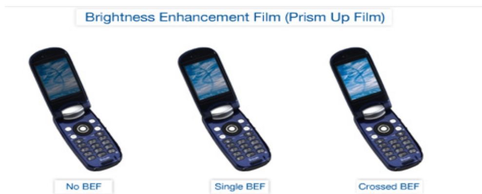
Figure 2.1.1.4 differences on the cell-phone screen with or without prism films.
