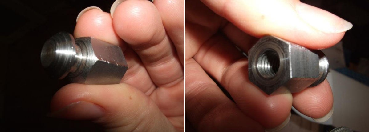
Figure 27 The existing adaptor for the RVA valve actuators
