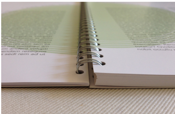
Figure 10.2 The spiral binding enables the pages in the assisting tool to remain laying open as the user desires.
