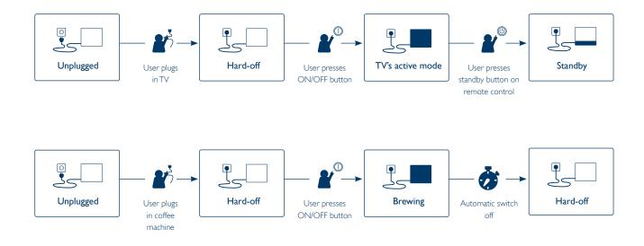
Fig. 4. Examples of power mode transitions. Top: a TV. Bottom: a dripfilter coffee machine
