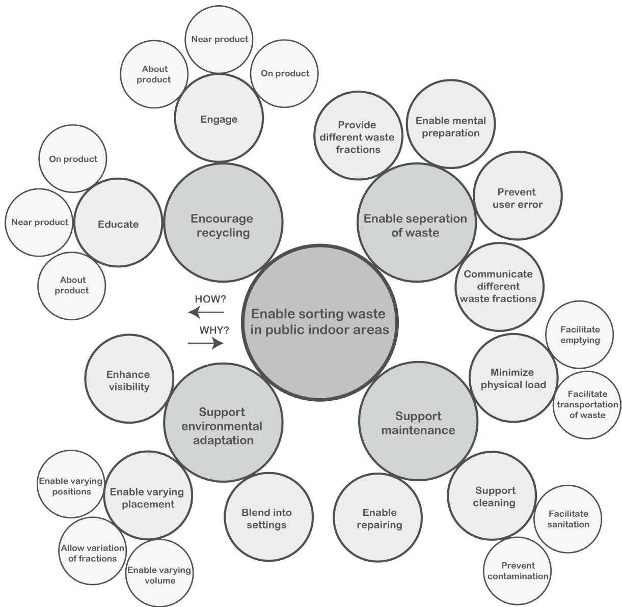
Figure 20. The function analysis with the main function, part functions, and support functions
