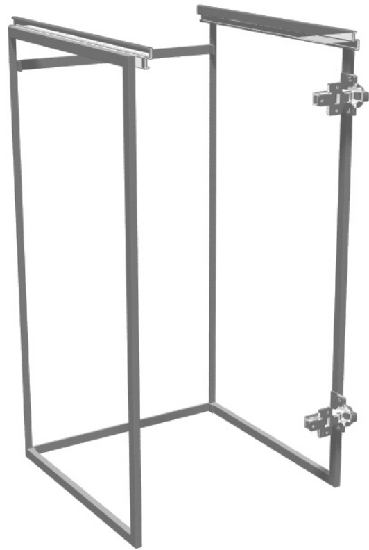
Figure 49. Hinges and rails could be fastened to the inner construction
