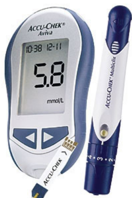
Figure 12. Shows that three components are needed to perform a test; blood glucose meter, lancet and test strip.
