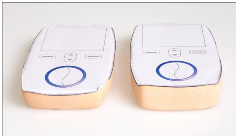
Figure 34. Two physical models used to evaluate and decide the design of the bottom and side surfaces.
