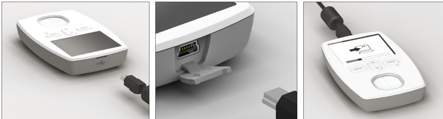
Figure 47. The procedure of connecting the meter to computer and/or external charger via the USB-port.
