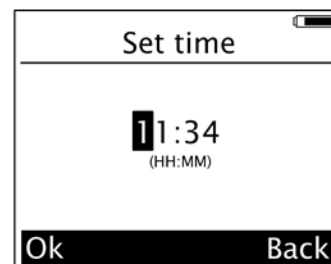
Figure 63. Set time screen. The black box marks the digit that is changed at the moment.
