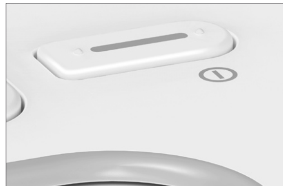
Figure 44. The right soft key with its navigation markers.
