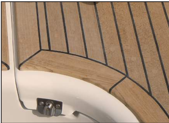
Caulk Teak Deck
