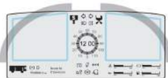
Two concepts with the most important information in the centre as a line with different placement of stop signals and time visualisation. Available information will be shown on the sides of the screen, making it available of showing two other information groups instead of one long one.
