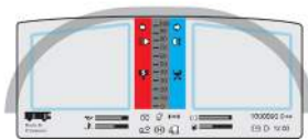
Available information on two sides with different visualisation of stop signals and speed. The idea is that the whole sides of the centre area will lit up with a red and blue colour if the stop buttons are used. Visualisation of the box could be taken away to make room for bigger visualisation of available information.
