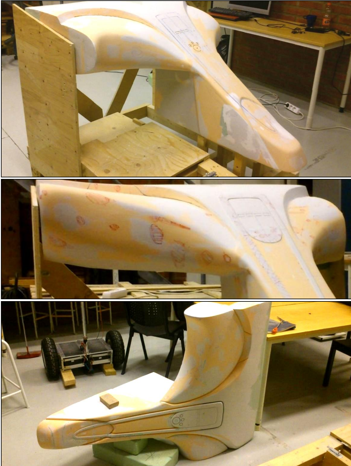
Image 57. Refining the shape and finishing the surface for prototype II
