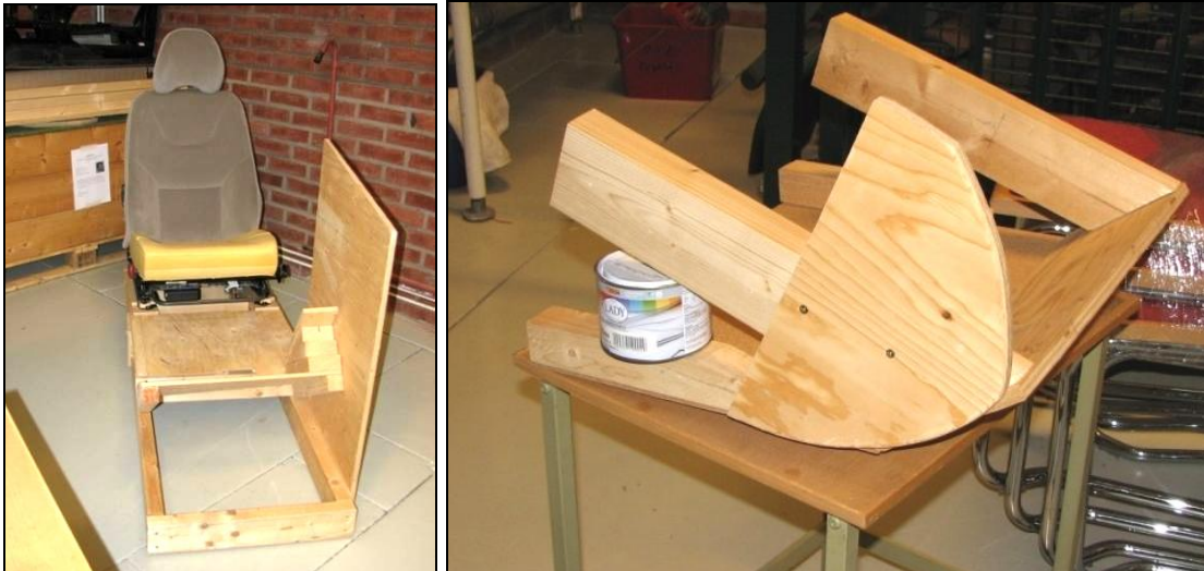
Image 48. The structure after removing the passenger-side limiter and steering wheel support
