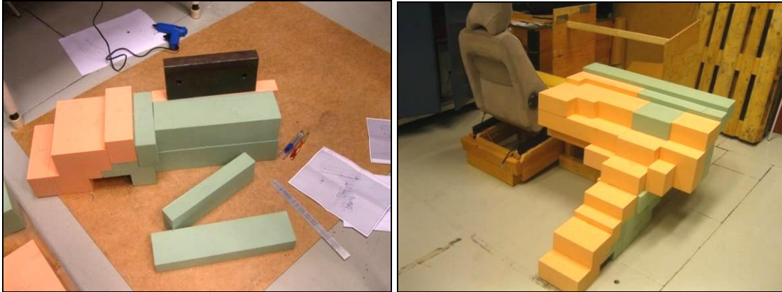
Image 54. Gluing the blocks to form the base of the dashboard
