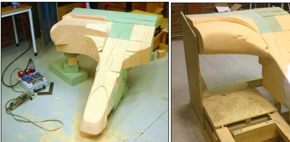
Image 56. Shaping the dashboard for prototype II
