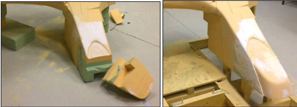
Image 62. Breakage during construction and after fixing
