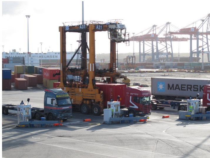
Fig. 4 Straddle carrier in the Skandia Harbor loading a 40 ft. container on a semitrailer
