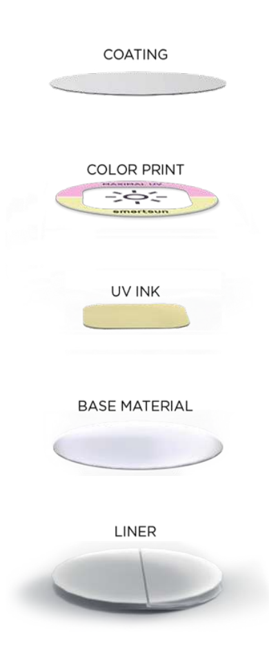
Figure 8.C. The patch's different layers
