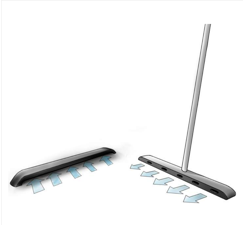
Figure 56 SUR - a suction device put beneath furniture and a stick blower.
