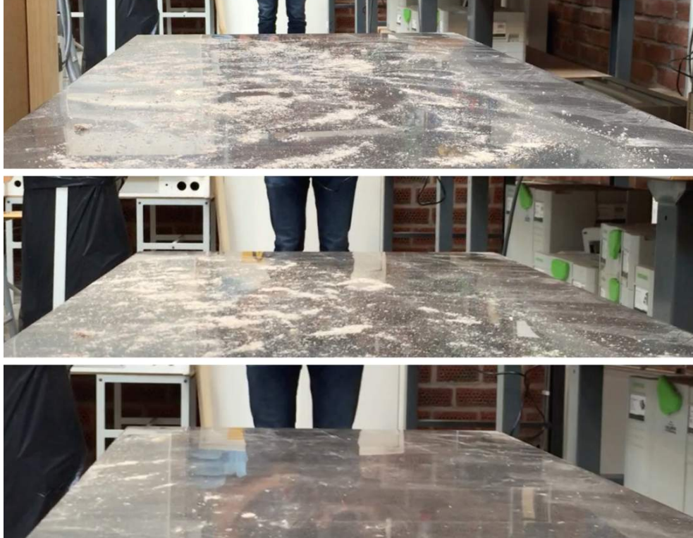
Figure 77 Dirt removed by blowing air from different distances, from top to bottom: 4-5 m, 3-4 m, 1.5-2.5 m.
