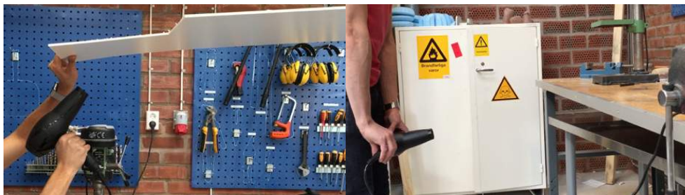
Figure 78 Blowing from below. Left: air does not “reflect”. Right: angled blowing can attach to a surface at higher heights.
