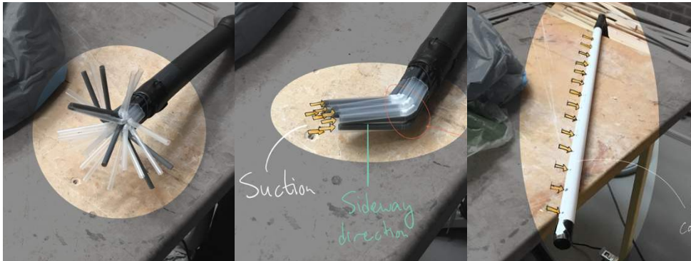
Figure 50 New suction nozzles, from the left: directed straws, spread straws, holes in a pipe.
