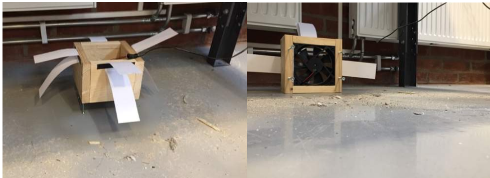
Figure 59 A prototype of Weasel. The paper strips were used as airflow indicators.
