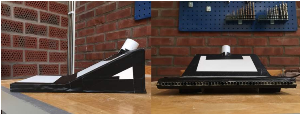
Figure 65 Modifications of the custom nozzle.
