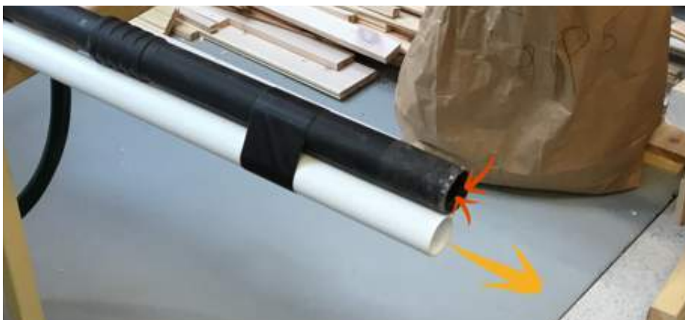
Figure 52 A blowing pipe attached to a vacuum cleaner pipe.
