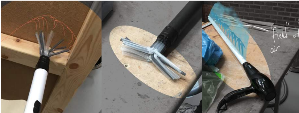
Figure 51 Different blowing nozzles, from the left: spread blowing, two-directional blowing, field of air.
