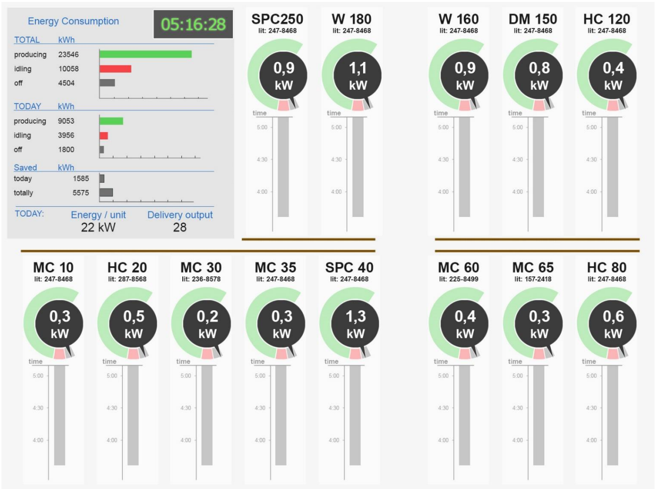
Figure 34. The appearance of the dashboard when every machine is turned off, at 05:16 in the morning in this image.
