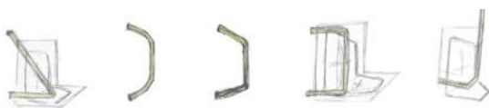
▼ Figure 43: Sketches of different handrails that were intended to be positioned adjacent to priority seats.
