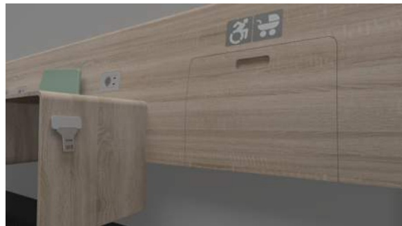
▲ Figure 67: Rendering of a simple safety belt buckle on the seat panel adjacent to the priority seat for wheelchairs and prams.
