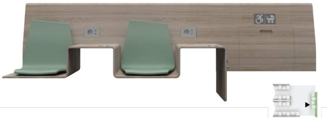
▲ Figure 72: The seating environment in the back of the cabin, with priority seating for either a wheelchair or a pram.
